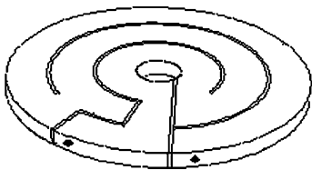
Fig. 2. Internal geometry of a cooled element within the CDCC.
